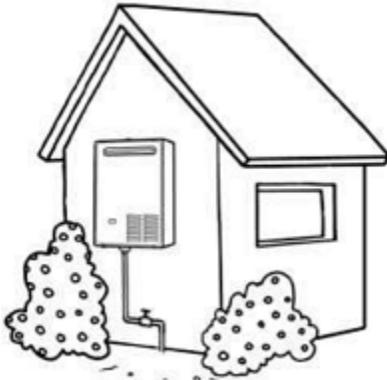
unit. Hot water is then plumbed from the unit into the existing or new reticulation supplying the premises. It is very important to ensure hot water piping is laid efficiently to reduce heat loss factors. The gas geyser units should be installed as close as possible to the point of highest hot water use.
